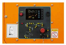
It has a base control and a platform control system that use commutation switches to convert. The basket control is used to lock the base control. The two systems are protected by shields.
